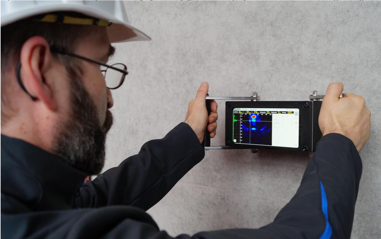
Figure 1: Ultrasonic tomography system for concrete testing
