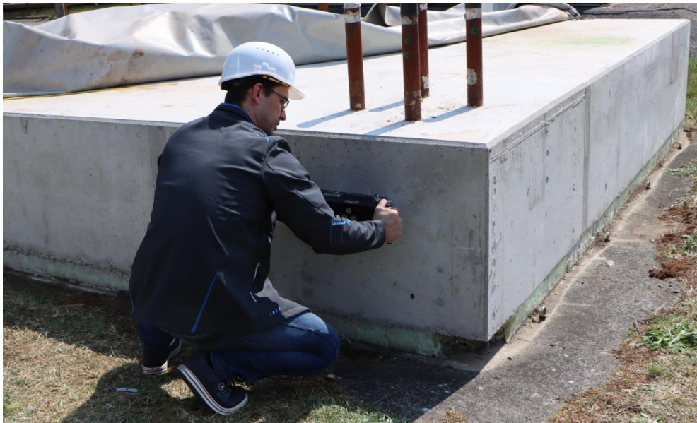
a) Measurements on a concrete block with a wall thickness of 4 m
