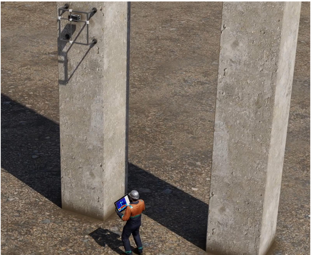
Figure 5: Possibility of an automated data acquisition via the wireless data interface
